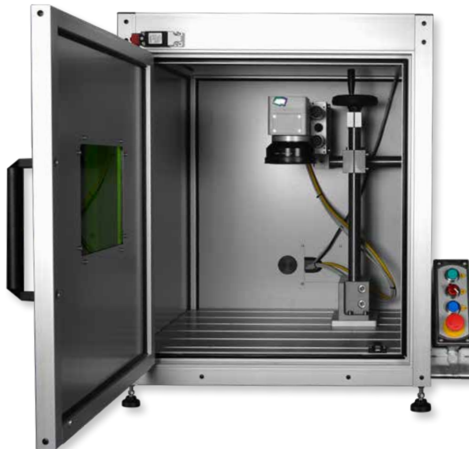
Viewing window and internal LEDs lighting. Vertical position adjustment for marking from above; it comes with handwheel and millimetric references
