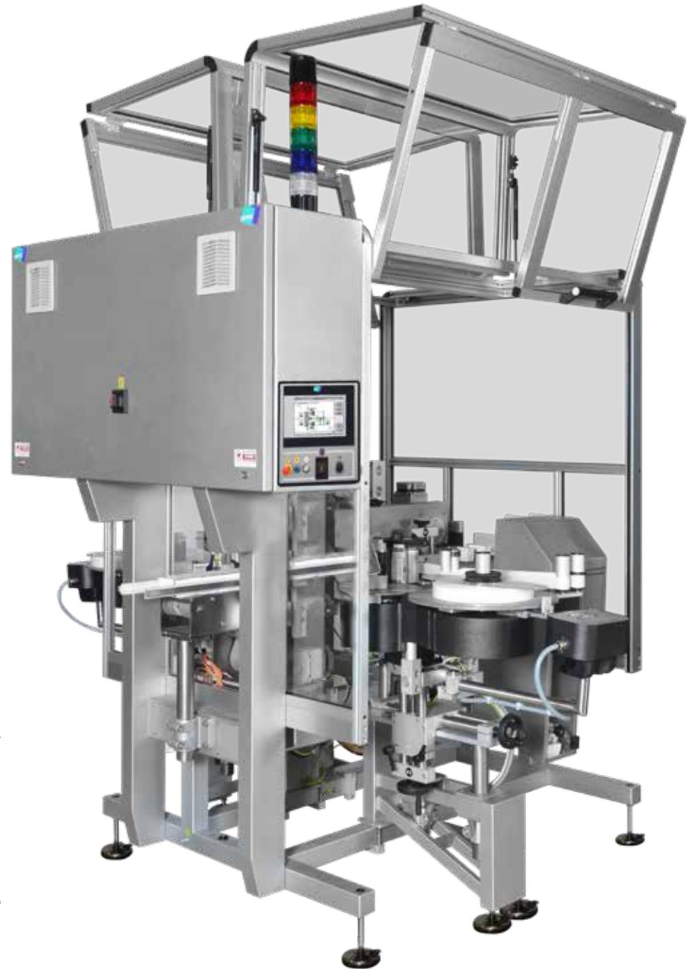
*Solid Skytech: the model with the "uplifted" electrical system cabinet, near the power supply. To wash and clean more freely.*
