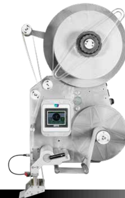
EVOLUTION 4.0 / PERFORMANCE 4.0 110/160/250/350 up to 80 m/min 262'/min 1200 pcs/min
