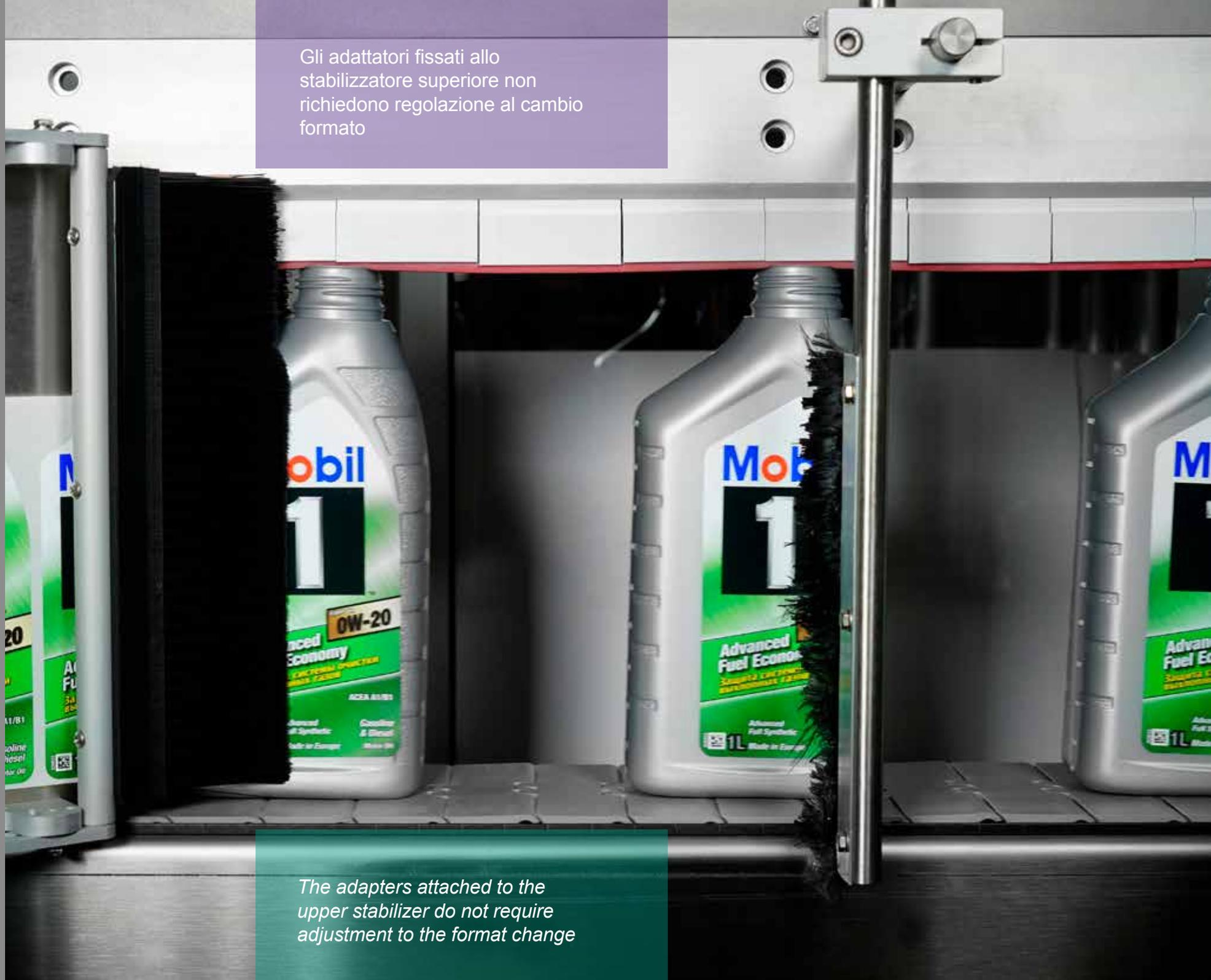
*The adapters attached to the upper stabilizer do not require adjustment to the format change*
