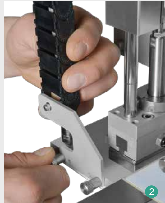
Couplings for rapid replacement of the label support pad (without employment of tools)
