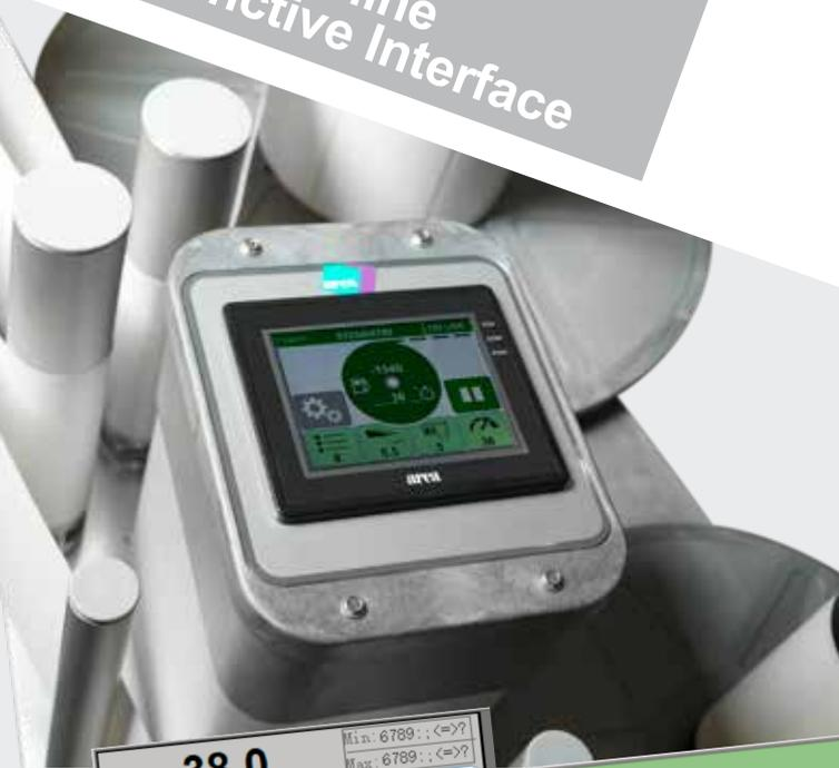
*Range Monitoring. Calculation in real time of autonomy, in pieces and in residual time (in performance function); with representation graphic / chromatic and display visualization of "approaching end of roll". The monitoring is always active, does not require any operation (fail proof). Requires the use of rolls whole labels or in any case with quantity of labels known*
