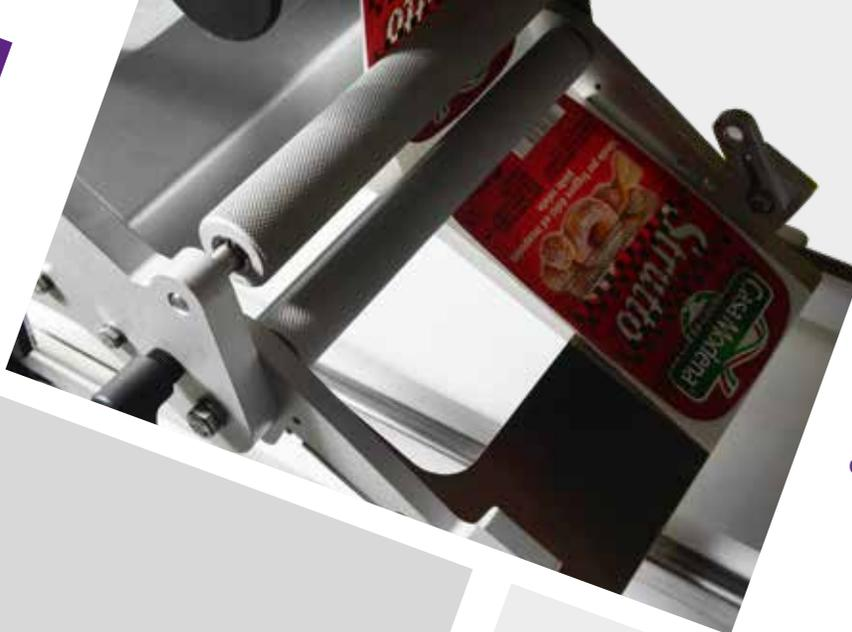
*The standard articulated peeler can also be used on flat surfaces, increasing safety thanks to its "mobility".
