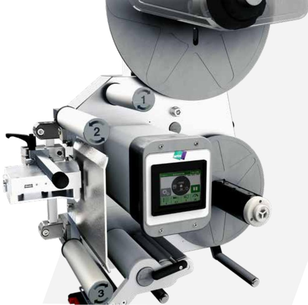
*The print head is set in the same cartridge, and is "HP compatible". Depleted cartridge replacements don't require any cleaning*
