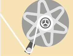
*Clever Rewinder. Motorized silicone support retractor with automatically adjusted speed according to the performance of the labeller (speed and frequency). It has no clutches to adjust and maintain*
